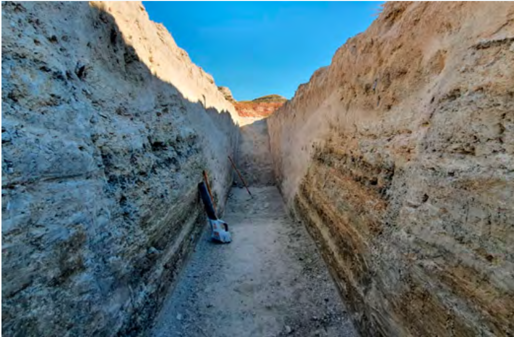
Figure 4. Interior of a palaeoseismic trench dug in the Galera fault to identify palaeo-earthquakes.
