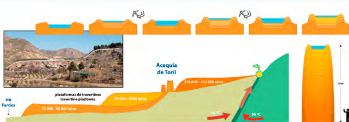
Figure 9. The figure explains how extraordinary this aqueduct is. Initially, human beings dug its channel several metres below its present level. The gradual accumulation of calcium carbonate in the channel, resulting from the special physical and chemical characteristics of the water, has caused the raising of the aqueduct and the formation in some areas of a wall up to 15 m high and over 4 m wide. According to scientists and datings made in the travertine of the aqueduct, its age, that is, the age at which the waters started to be diverted and the wall on which the water runs today began to form, is over 3,000 years.
